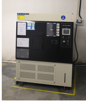
Aging test chamber (Xenon lamp)
