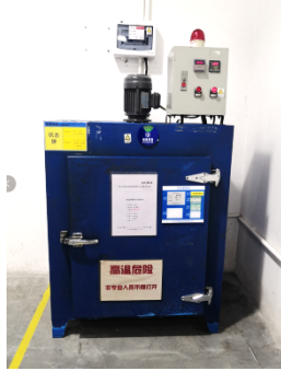
Aging test chamber (High temperature)
